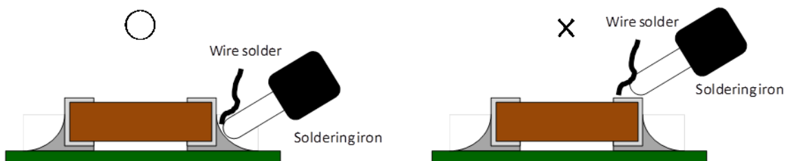
Fig 3 Correct handling method of soldering iron
